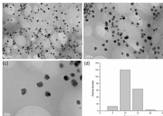
**Fig. 2:** TEM micrographs at different magnifications (a-c) and size distribution (d) of AgNPs
