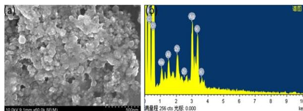
**Fig. 3:** SEM micrograph (a) and EDX spectroscopy (b) of AgNPs
