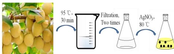
**Scheme 1:** Schematic diagram of AgNPs synthesis
