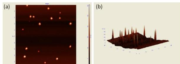
**Fig. 4:** AFM images of AgNPs synthesized by ginkgo fruit extract: (a), morphological feature of the nanoparticles; (b), 3D topographic view of the nanoparticles
