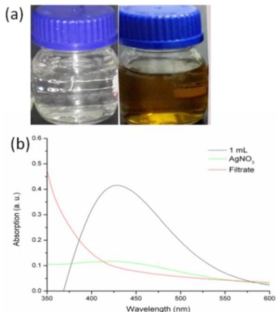
**Fig. 1:** Green synthesis of AgNPs, based on 1 mL ginkgo fruit extract: (a), color change of diluted filtrate before and after adding 1 mM  $\text{AgNO}_3$  at  $80^\circ\text{C}$ ; (b), UV-Vis spectrum of AgNPs
