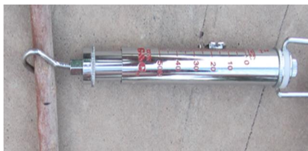
Fig. 3: Mapping of normal forces given by tension meters (resistance forces to plants)
