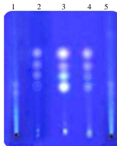
Fig. 3. Effect of origin green coffee beans on detection of aflatoxins using the AOAC method. 1, Aflatoxins-free-Brazilian coffee beans; 2, Spiked Brazilian coffee beans with aflatoxins; 3, Aflatoxins standard; 4, Aflatoxins-free-Colombian coffee beans; 5, Spiked Colombian coffee beans with aflatoxins; 6, Aflatoxins-free-Ethiopian coffee beans; 7, Spiked Ethiopian coffee beans with aflatoxins.
