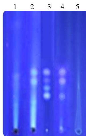
Fig. 7. Effect of processing coffee beans on detection of aflatoxins using an improved procedure. 1, Aflatoxins-free Colombian roasted coffee beans; 2, Spiked-Colombian roasted coffee beans with aflatoxins; 3, Aflatoxins standard; 4, Spiked-Colombian decaffeinated coffee beans with aflatoxins; 5, Aflatoxins-free Colombian decaffeinated coffee beans.
