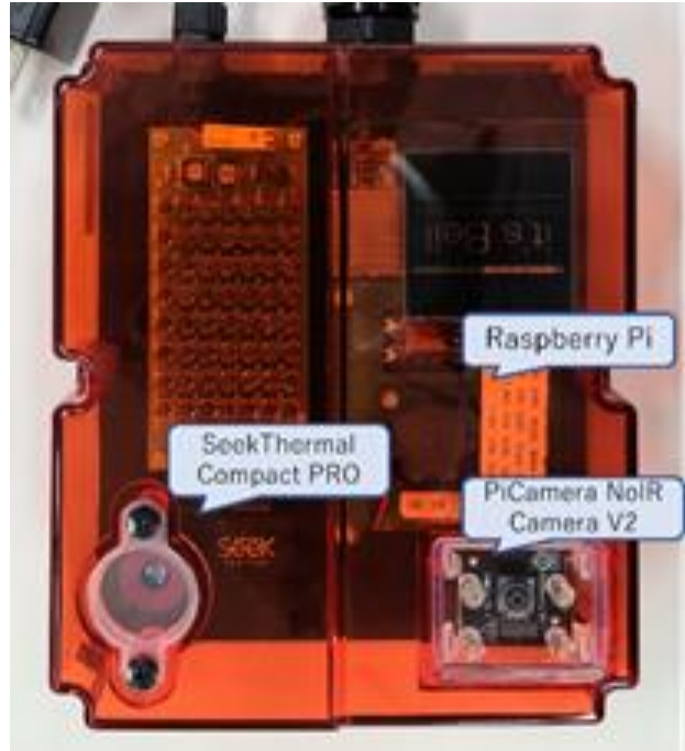
Fig. 3: Device used in experiment: Raspberry Pi, visible light and infrared camera
