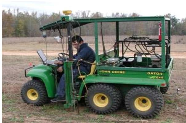
**Fig. 2. The control system for variable-depth tillage operations**
