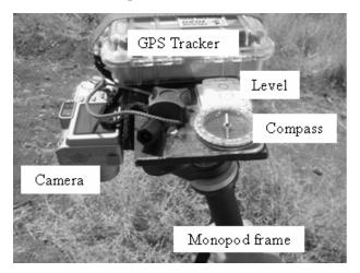
Fig. 2: Both oblique (top) and vertically downward (bottom) images are taken in the field with the staff mounted digital cameras
