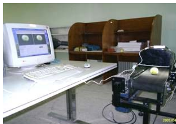
Fig. 5. Automatic data acquisition system used for apple grading
