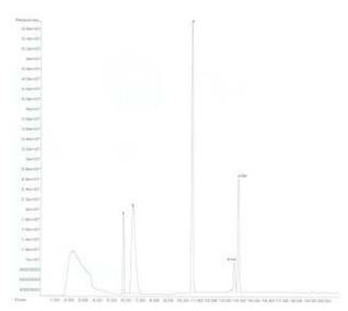
Fig. 4. Separation of four pesticides in wheat grain fortified at 0.1 mg/kg quantifying on a 30 m HP-5 MS capillary column, Peaks: 1. malathion, 2. chlorpyriphos, 3. bifenthrin and 4. permethrin (a, b)
