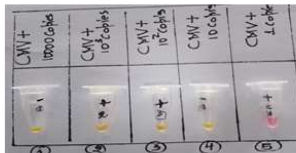
Fig. 4: The LAMP method developed in this study can detect an extract containing >10 copies/tube or >150 IU/ml
